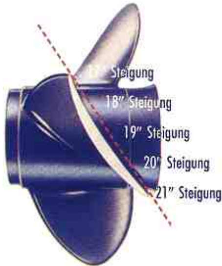
progressive Steigung (pitch)
