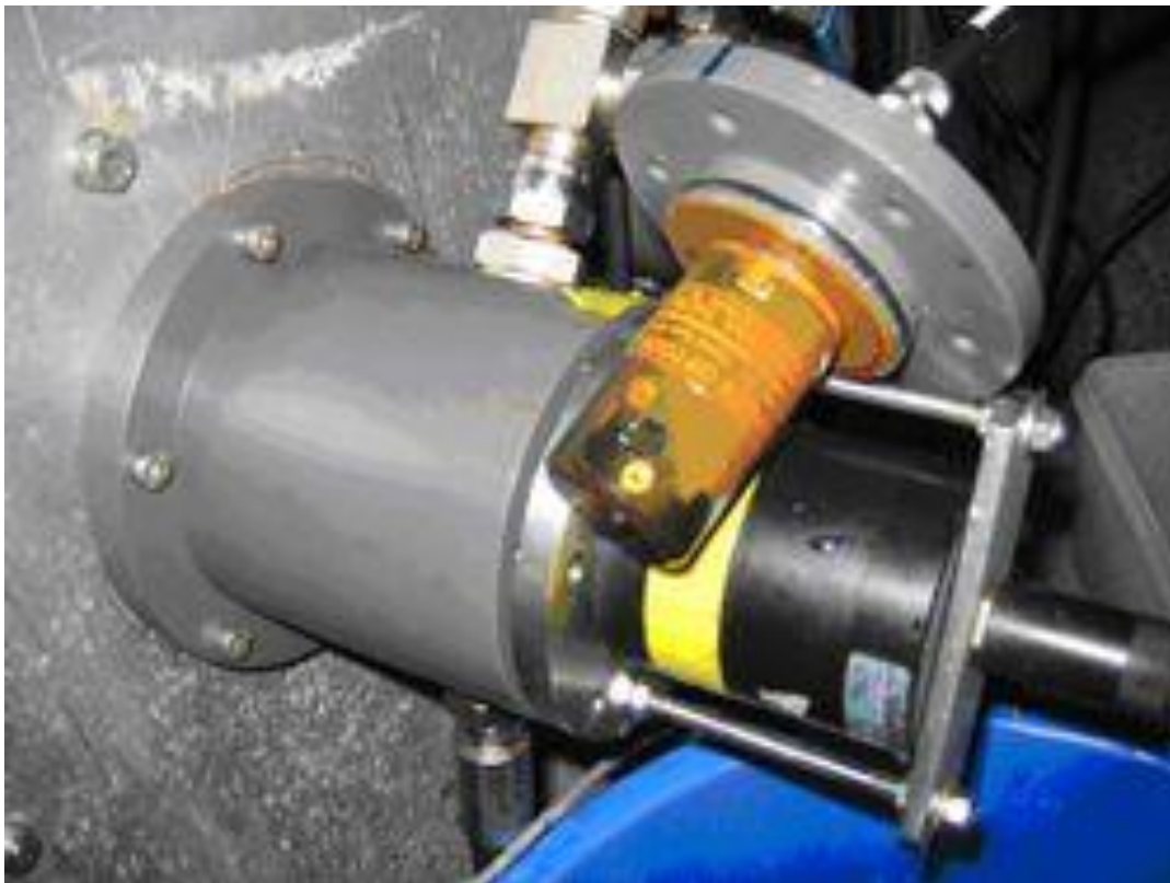
Fig. 2: Photographs of the Aanderaa optode removed from its housing for cleaning
